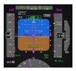
You should be prepared to disconnect the auto throttle during flare, which you can do either with the A/T ARM switches on the Glareshield MCP, or with the side button on the throttles. If using the side button on the throttles, first highlight the throttles and then left click to view the button clicking options for the throttles with tooltips on.
