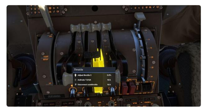
Now you are ready to begin your takeoff. Confirm your PFD FMA shows TO/GA - TO/GA for roll and pitch modes and that your auto-throttle arm switches are on. To engage the auto-throttle to set takeoff power, you will need to press the TOGA button once (or use a control binding for AUTO THROTTLE TO GA). If using the click spot on the throttles, first highlight the throttles and then right click to view the button clicking options for the throttles with tooltips on.
